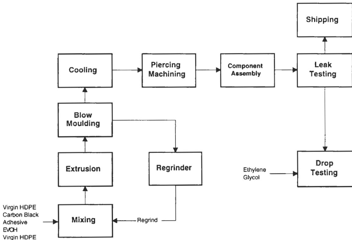
**Figure 3-2 Multilayer Plastic Fuel Tank Manufacture**
