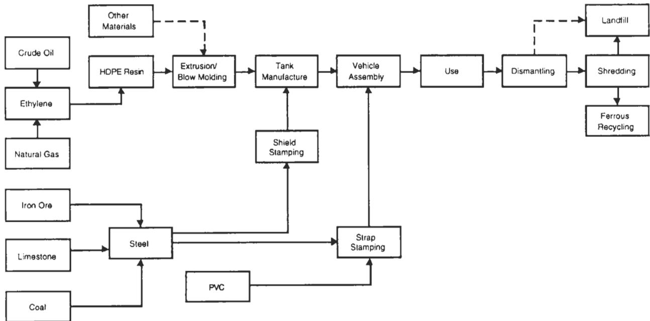
Figure 2-3. HDPE Fuel Tank System
