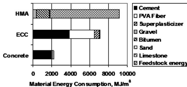
Fig. 4. Primary energy consumption per volume of each material
