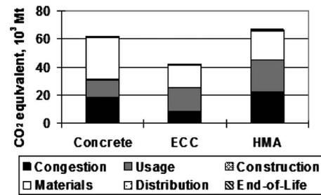
Fig. 7. Greenhouse gas emission by life-cycle phase
