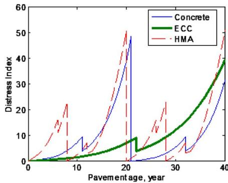
Fig. 5. Distress index of each pavement
