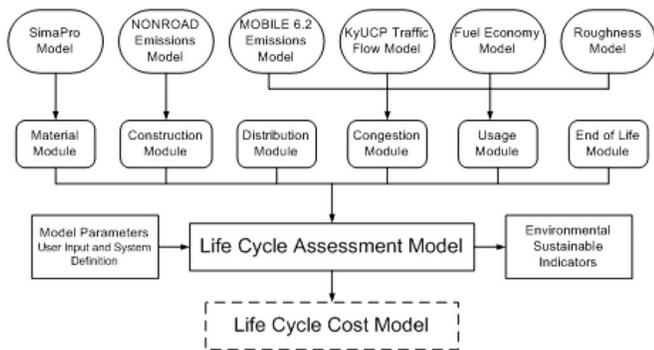
Fig. 3. Logic relationship between LCA component
