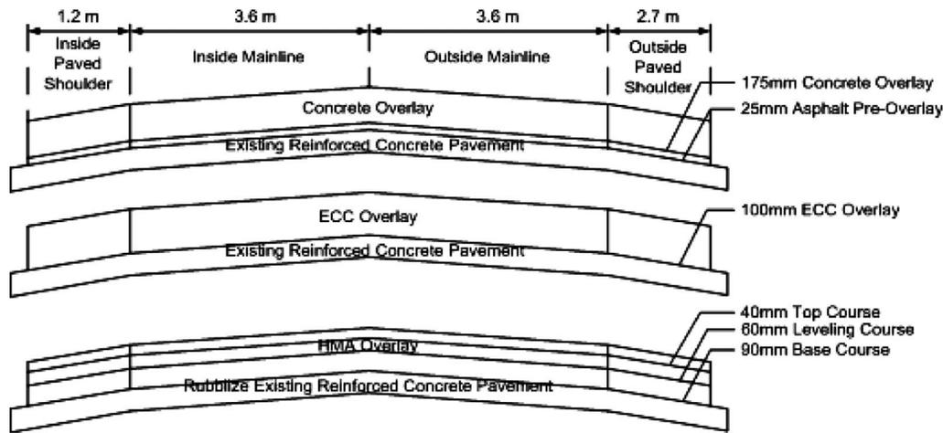
Fig. 1. Overlay structure and thickness in one direction
