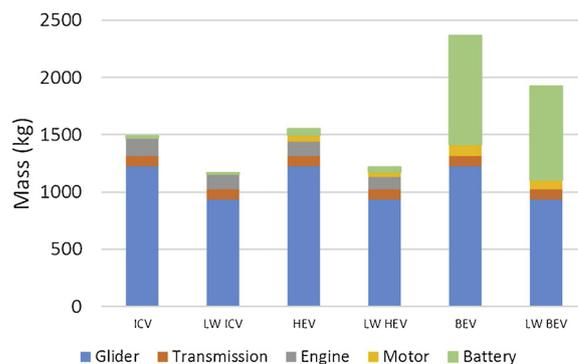
Fig. 2. Mass specifications of vehicle components [51].
