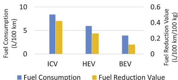
Fig. 3. Fuel consumption and fuel reduction values across powertrain types [51].
