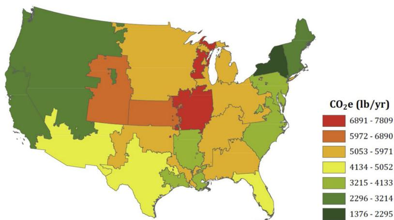
Fig. 4. Annual GHG emissions of Ford Focus BEV. The comparison value for a Focus ICEV is 9557 lb/yr [78,79].
