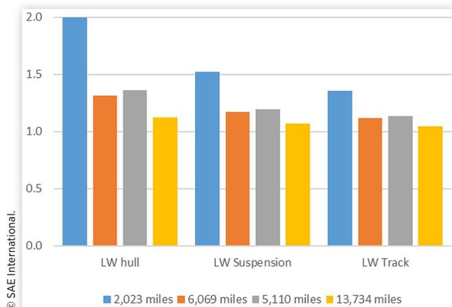
**FIGURE 5** Fractional costs for upgrading the M1A2 with lightweight components over duty cycle 3 over 3 decades
