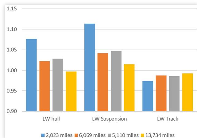
**FIGURE 7** Relative cost values ( $B_{LWT}/B_{OMT}$ ) for refurbishing/refitting and operating an LWT over various DSTs
