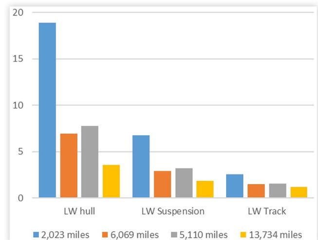
**FIGURE 3** Relative fuel use ( $B_{LWT}/B_{BCT}$ ) for the LWT over the BCT operated over various DSTs
