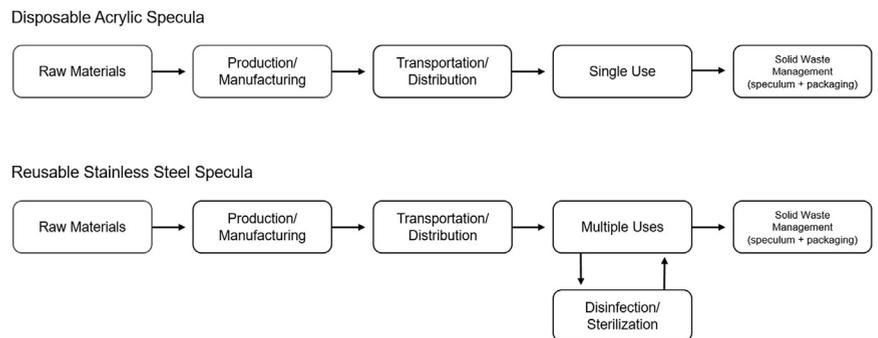
The diagram details the aspects of the speculum life cycle that is included in this analysis, which includes production, manufacturing, use, and disposal.
