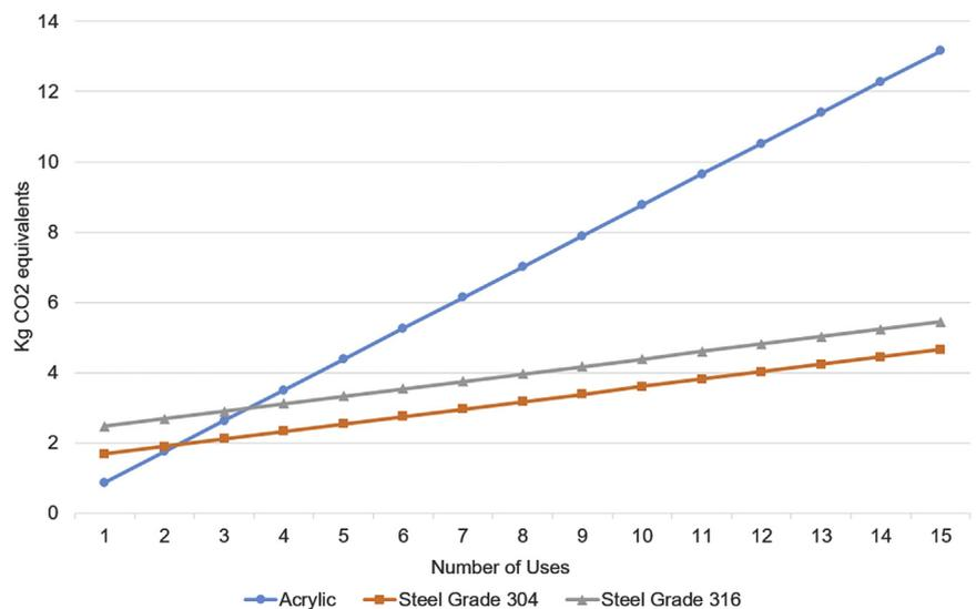
For data for the stainless steel specula, we assume sterilization in a half-loaded autoclave run on the ReliabilityFirst Corporation grid.
